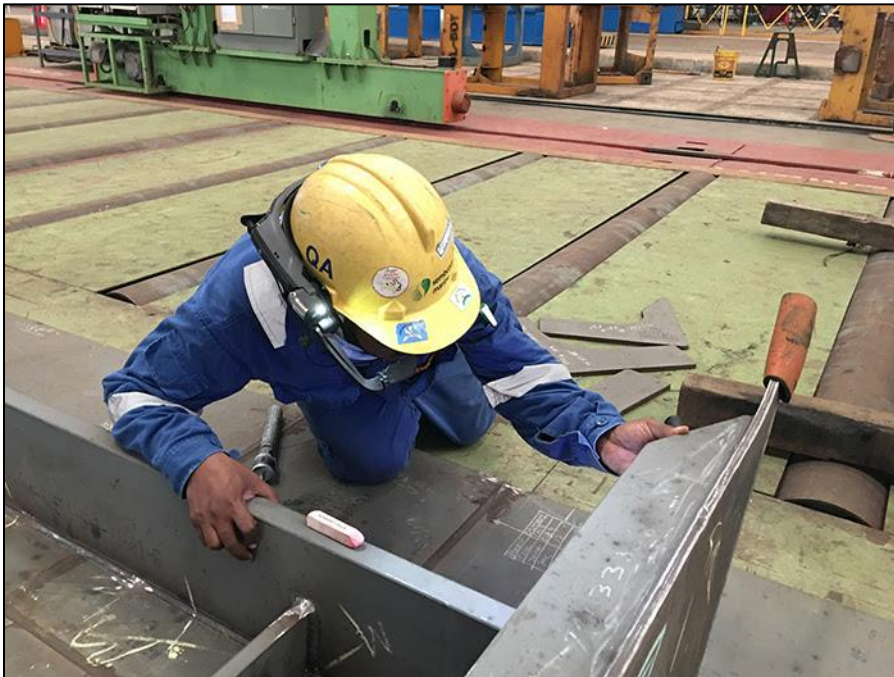
Sembcorp Marine Quality Control inspector working with helmet-mounted camera and communication device
