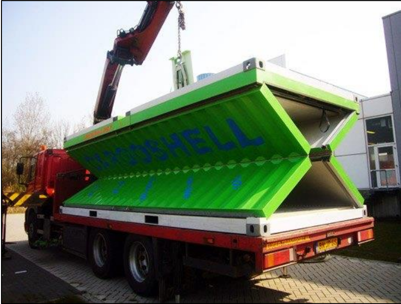
Cargoshell Containers. Made up of composite materials and with roll-up doors. Image marineinsighte.com
