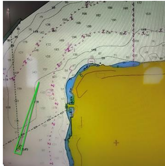
Figure 2: A representation of an AIS broadcast for a towing vessel pushing a 1,600' tow, properly entering overall dimensions, and using Ship Type 57. (Actual view may vary based on type of Electronic Charting System and chart scale, as
