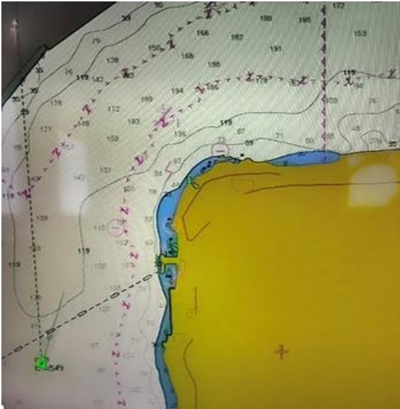
Figure 1: A representation of an AIS broadcast for a towing vessel pushing a 1,600' tow, and using Ship Type 31 (Actual view may vary based on type of Electronic Charting System and chart scale as set by user).
