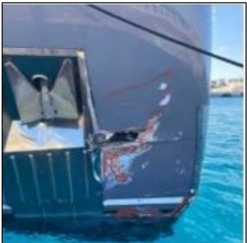
Utopia IV bow damage
