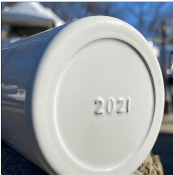
Fire extinguisher date stamp
