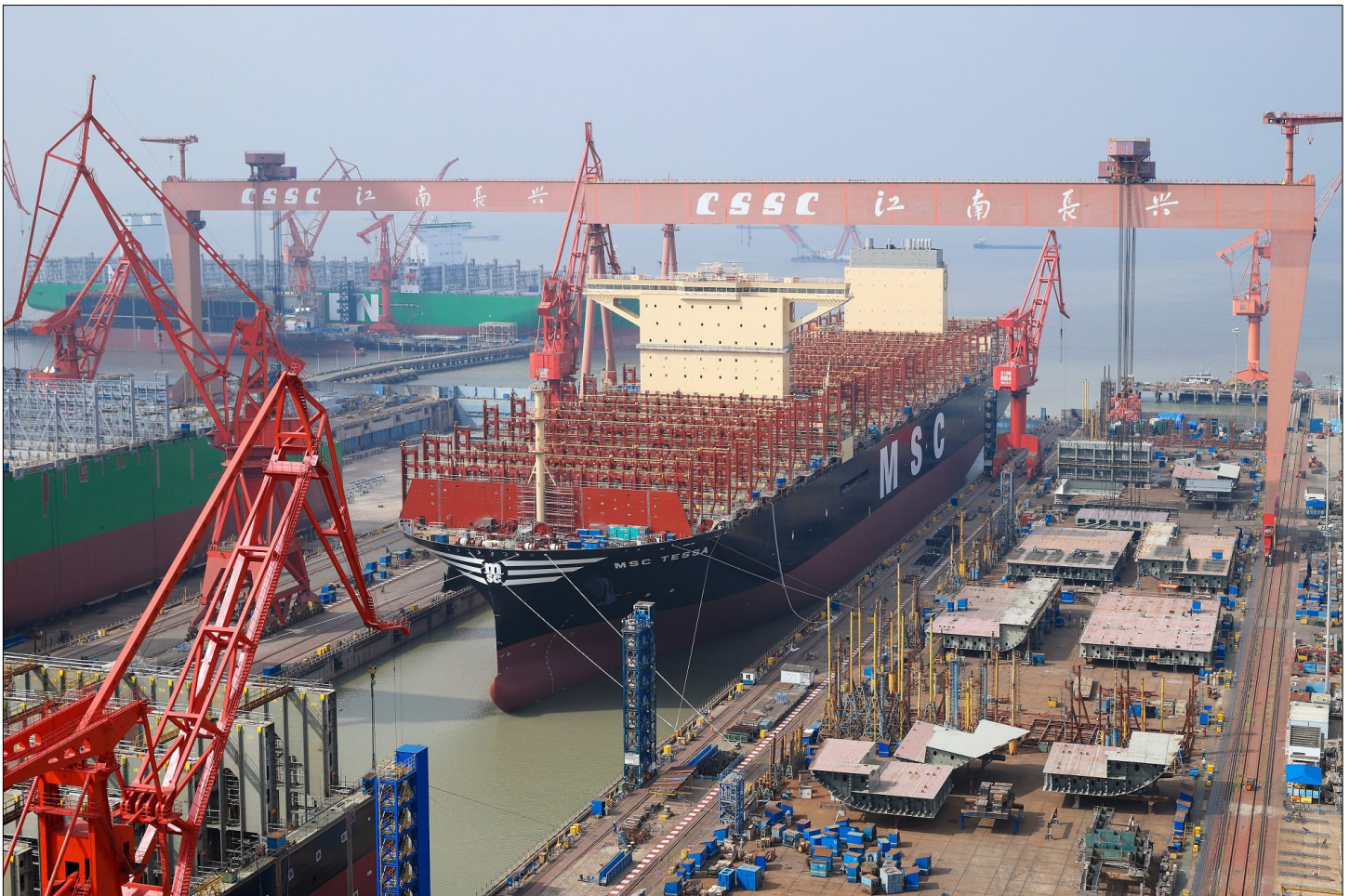
Figure 19: MSC Tessa, one of the world's largest containerships, under construction at Hudong-Zhonghua Shipbuilding in Shanghai, China. Photo courtesy CSSC.
