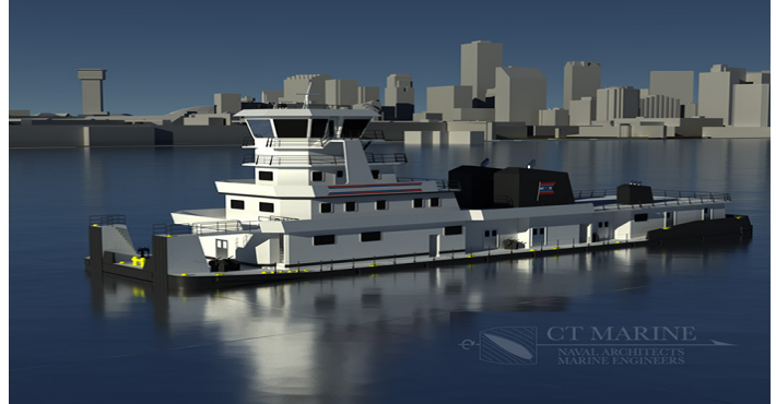
Figure 5: On delivery, the 11,000 hp towboat will operate on ACBL's mainline network pushing up to 56 barges, averaging approximately 75,000 tons of cargo.
