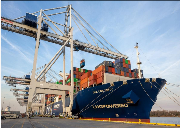
Figure 15: Electric ship-to-shore cranes work the CMA CGM Unity, powered by liquefied natural gas, at the Port of Savannah's Garden City Terminal. Credit: Georgia Ports Authority / Emily Goldman
